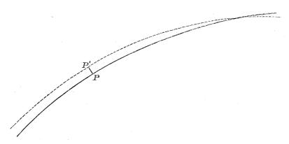
Take a point P on the mean surface and let the normal at P meet the surface of the distorted body in P'.
